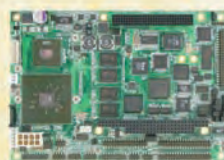
POSEIDON EPIC SBC Integrated CPU and data acquisition
