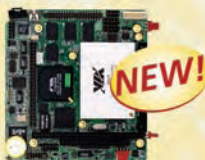
ATHENA II Compact PC/104 SBC High performance in small package
